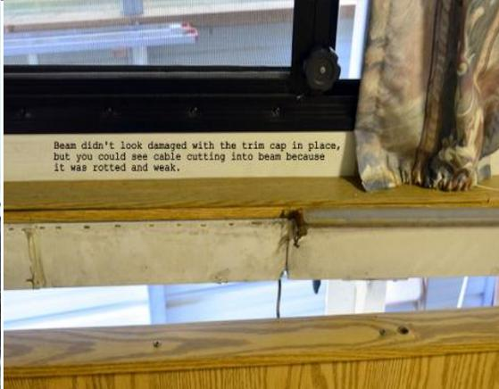
The last photo above on the right is showing the top and bottom halves of the camper separated and the aluminum covered beam at the bottom of the upper half. The lift cable cut through the aluminum beam cover because the beam was rotted and weak.
