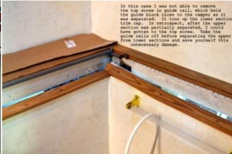
In this case I was not able to remove the top screw in guide rail, which held the guide block close to the camper as it was separated. It tore up the lower section trim cap. In retrospect, after the upper section was partially separated, I could have gotten to the top screw. Take the guide rails off before separating the upper from lower sections and save yourself this unnecessary damage.
