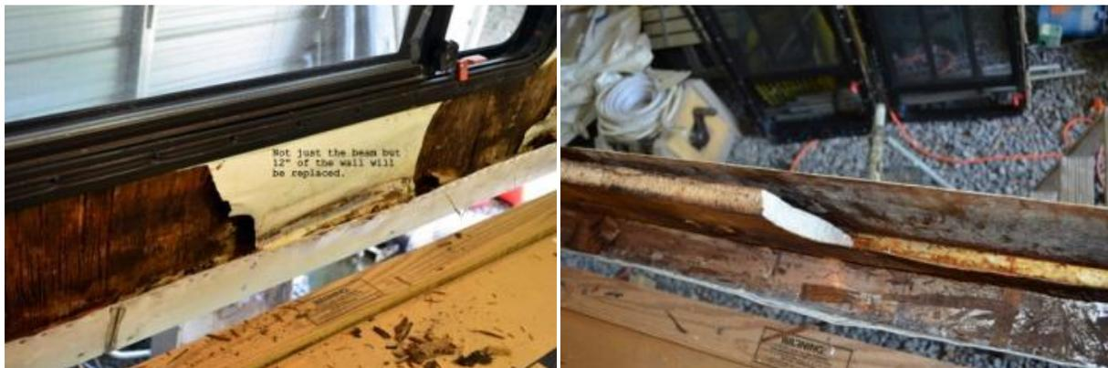
You can see in the photos above that the composite camper wall, consisting of 1/16" fiberglass outside skin, 1/8" plywood, 1" of foam, and 3/16" plywood inner wall was rotted and delaminated below the windows. The photo on right is looking down into the wall where a window was removed, with the rotted wood beam and portions of the wall also removed. The remainder of the 1" foam insulation below the window opening in the photo will be removed to rebuild the wall.
