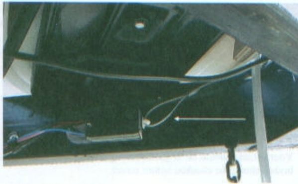
Figure b. Break-Away Switch
