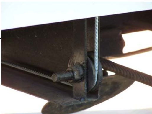
Lift pulley where cable goes into trailer wall to upper pulley
