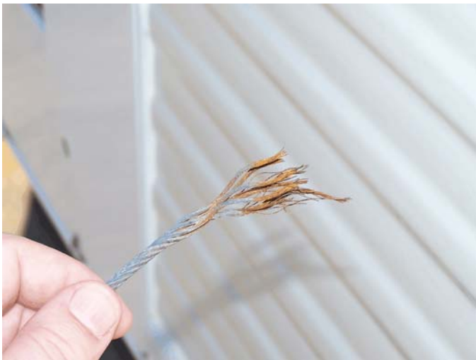
This is the one that broke first! Rust weakened the strands of steel cable to the point of failure.
