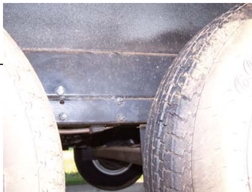
My adjustment & jamb nuts in frame
