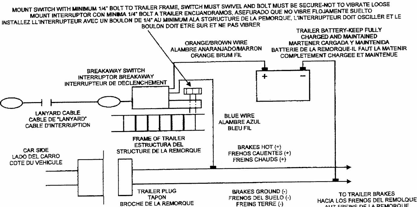
ALL WIRE CONNECTIONS SHOULD BE SECURE AND PROTECTED FROM CORROSION AND MOISTURE
