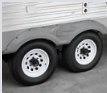
AL-KO Ultralube axles and 15" Radial tires are standard on all models.
