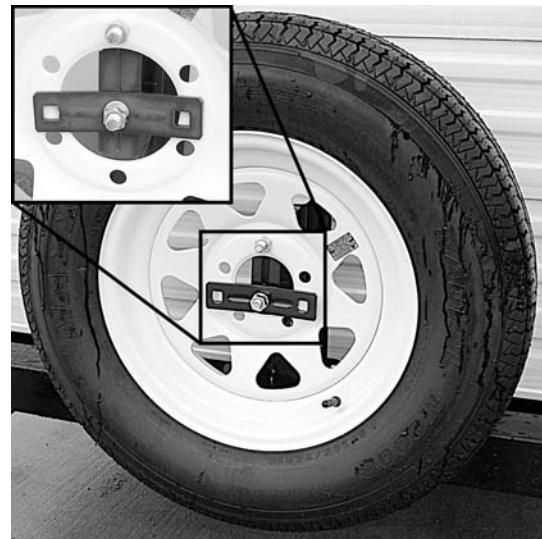
Fig 6.5 Spare tire carrier installation
