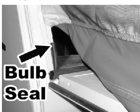
Fig. 8.5 Bulb seal
