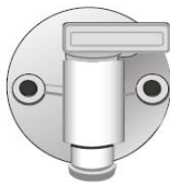
Fig. 8.8 Exterior fresh water drain
