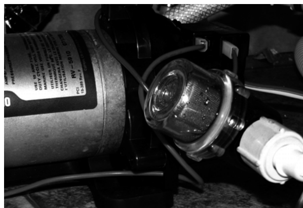
Fig. 7.3 Water pump strainer
