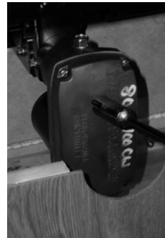
Fig. 10.6 M-Tec crank handle inserted to override the slideout motor
