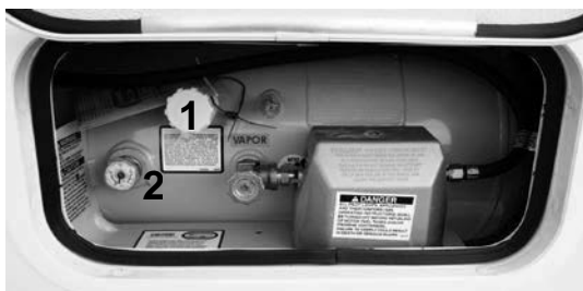
1: Propane fill valve; 2: Propane gauge
