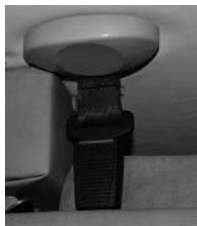
Fig 12: Belt Interlock Latched
