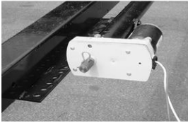
Fig. 3-Hex Head Crank Extension
