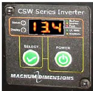
**NOTE:** When in Inverter Mode you will be able to cycle through Battery Voltage, Inverter Power, inverter settings and error codes. When in Bypass Mode you will be able to cycle through Battery Voltage, inverter settings and error codes. Inverter Power will not be available because the inverter is idle.
